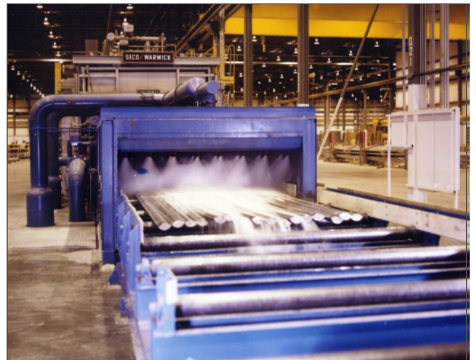
Solution Heat Treat Furnace with Spray Quenching for aluminum extrusions
