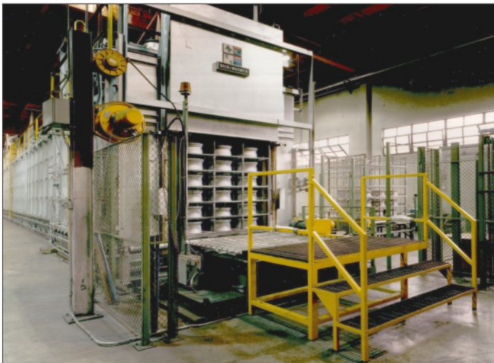
Fully automated solution heat treat and aging system for automotive wheels
