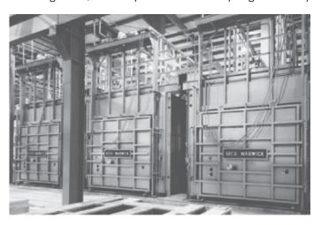
load configuration. In very large coil applications and where tight temperature tolerance is required, SECO/WARWICK designates two temperature-control zones for each recirculation fan. This field-proven design compensates for differing coil characteristics, combustion performance, and loading practices.
