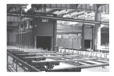
of the coil or even fatal degradations by local melting of the coil surface. The reason for these degradations is local overheating at the coil head surface caused by non uniform heat flow of the convective heat transfer system used.
