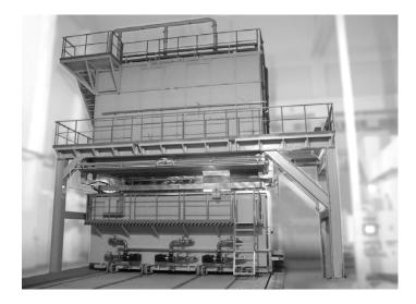
This innovative AMS compliant technology enables very fast and full load immersion as short as 5 seconds. As the VertiQuench name implies, the process provides very fast vertical quenching. The heat-treated material is dropped into water or polymer quenching tanks located directly under the furnace.
