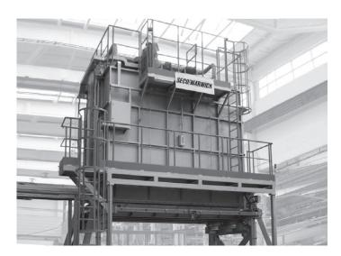
VertiQuench provides an optimal heat treatment technology for aluminum alloy extruded and drawn porthole or seamless tubes of 2xxx, 6xxx, and 7xxx series alloys in hard tempers, since it provides the shortest quenching time and produces the highest mechanical properties of treated extrusions.
